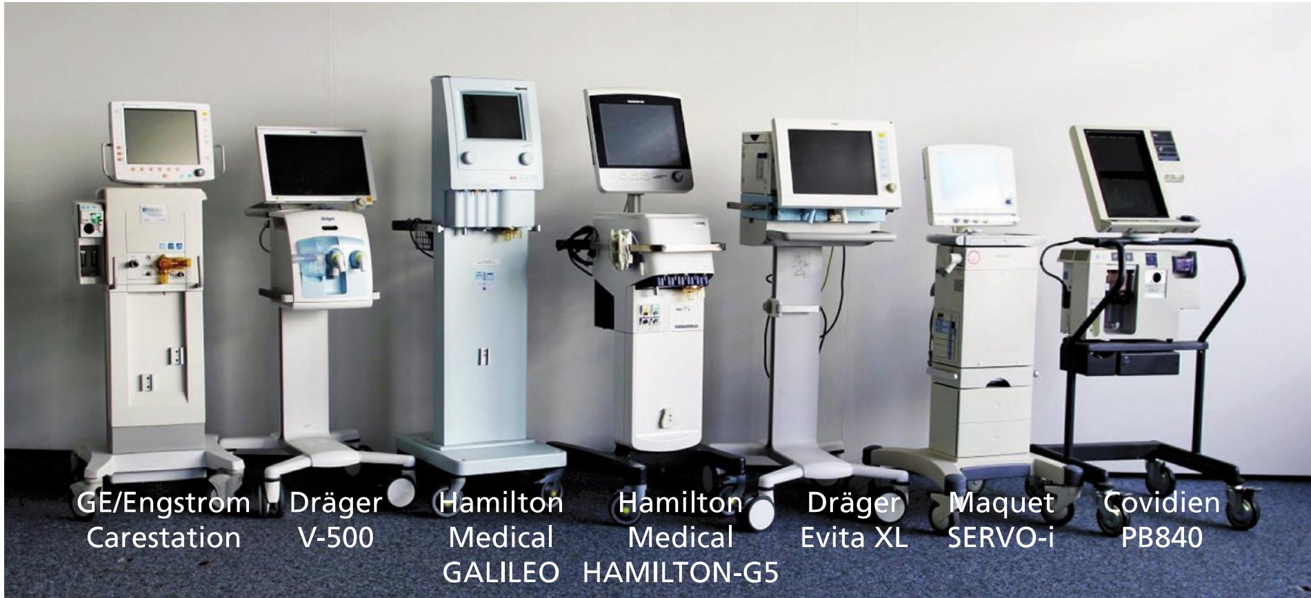
Fig. 3.13 Some popular ICU ventilators based on the intermittent positive pressure ventilation (IPPV) principle.
